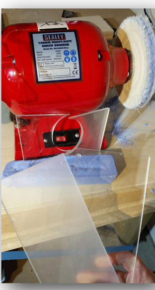
Light-diffusing pattern was buffed off of the acrylic
