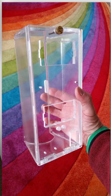
Light-diffusing pattern was buffed off of the acrylic
