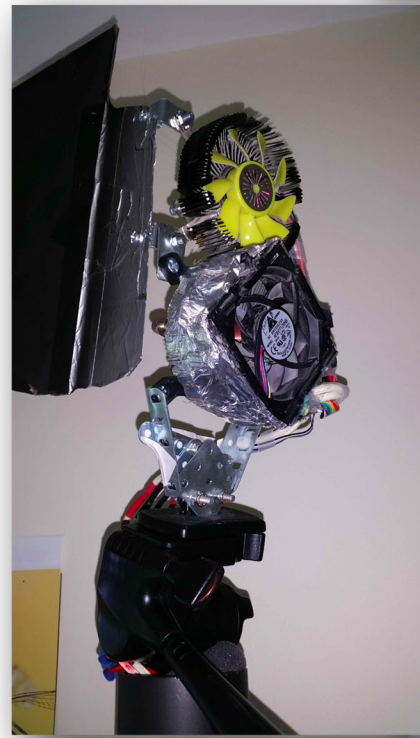
LEDs cooled by 2 CPU fans attached to pan-tilt head and light-blocker card using brackets
