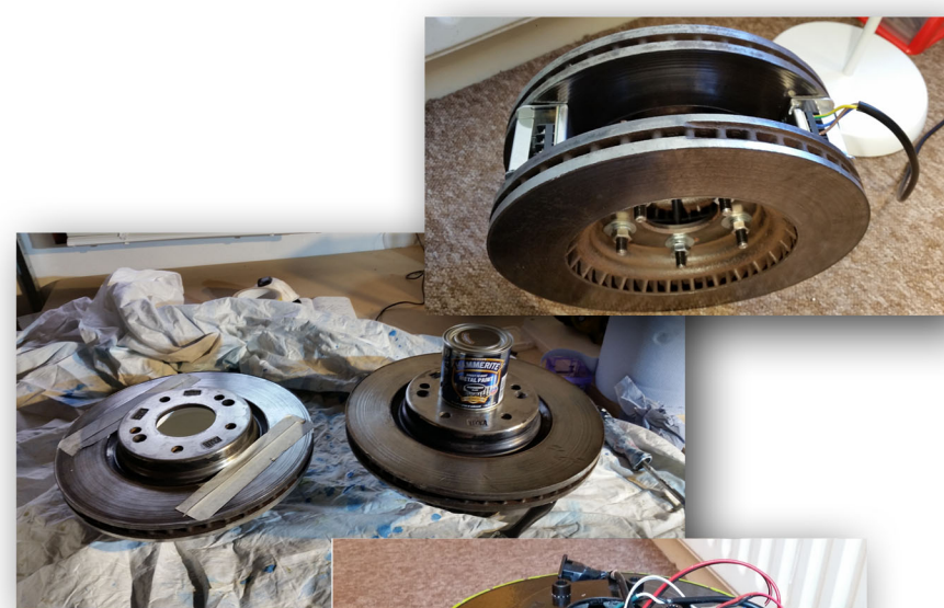
Two power supplies clamped between two heavy brake disks, painted and covered with fluorescent acrylic panels cut on the Handibot
